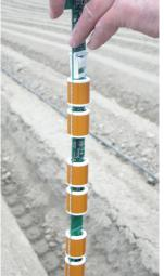
First probes are installed to establish soil moisture readings.
